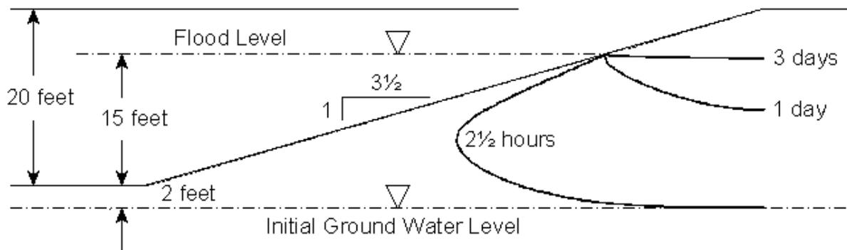
Figures 2: Position of the zone of saturation as a function of time, with the water level in the channel at flood stage, for a soil permeability of  $10^{-3}$  feet per minute.
