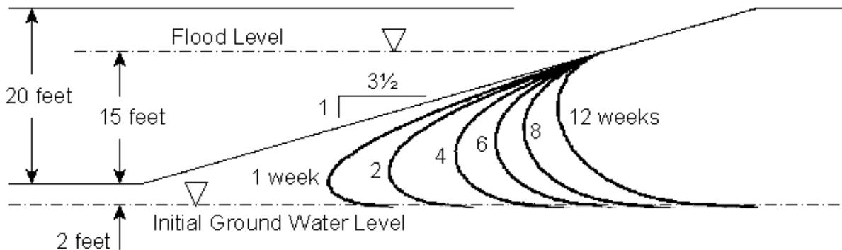
Figures 3: Position of the zone of saturation as a function of time, with the water level in the channel at flood stage, for a soil permeability of  $10^{-6}$  feet per minute.
