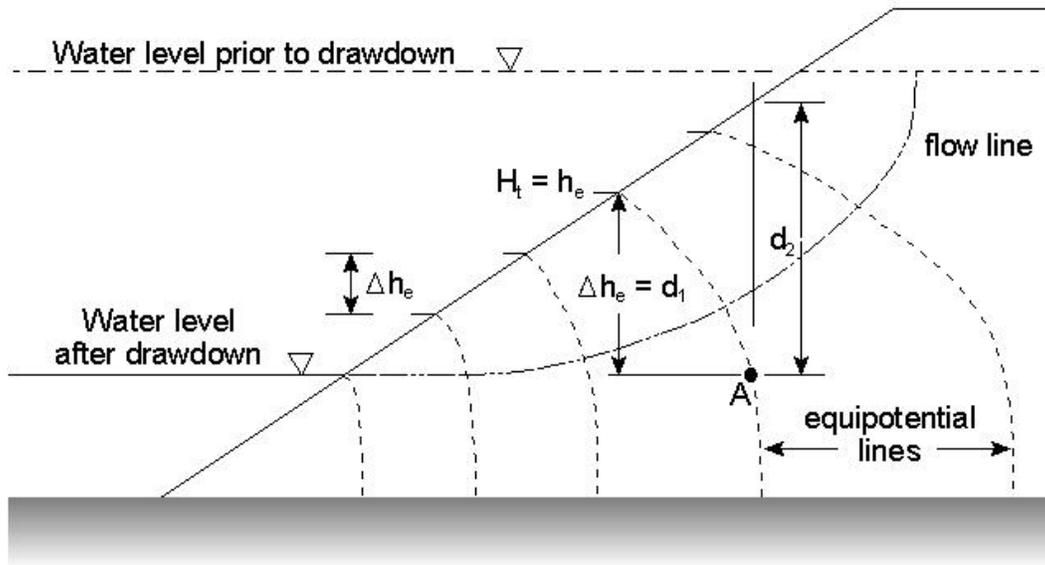
Figure 1: Flownet for a saturated slope after instantaneous drawdown.
