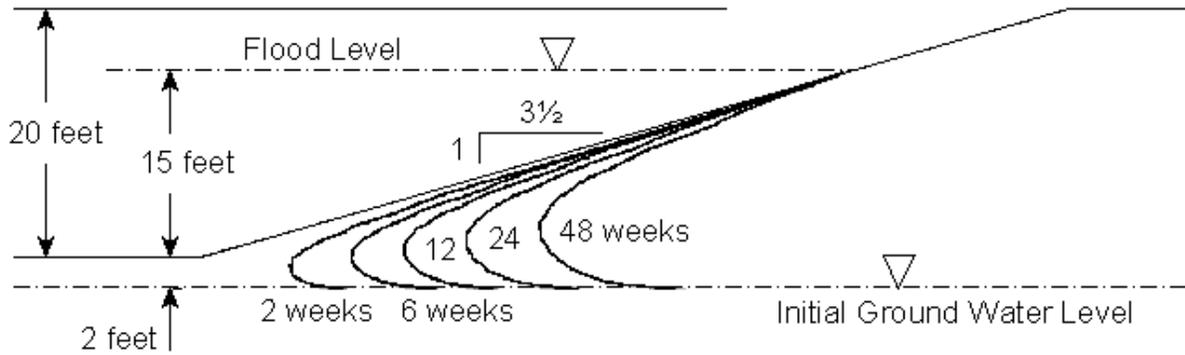
Figures 4: Position of the zone of saturation as a function of time, with the water level in the channel at flood stage, for a soil permeability of  $10^{-8}$  feet per minute.
