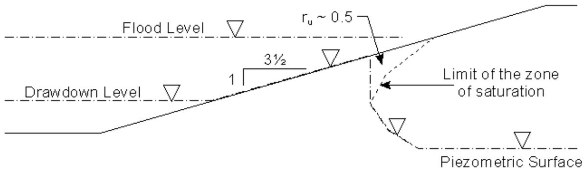
Figure 5: Illustration of the use of a pore pressure ratio and piezometric surface for a rapid drawdown slope stability analysis.
